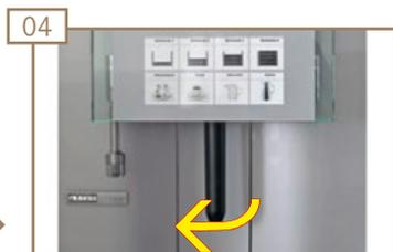
04 Turn the outlet tube clockwise by approx. one quarter of a rotation.
